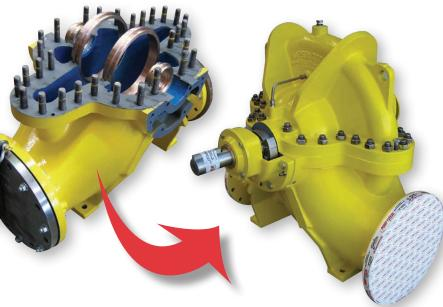
After receiving and disassembling an item of equipment or pump into our service centre, a full report of its condition will be produced. When repairing a machine to "as new" or including improvements, the following points are addressed:
